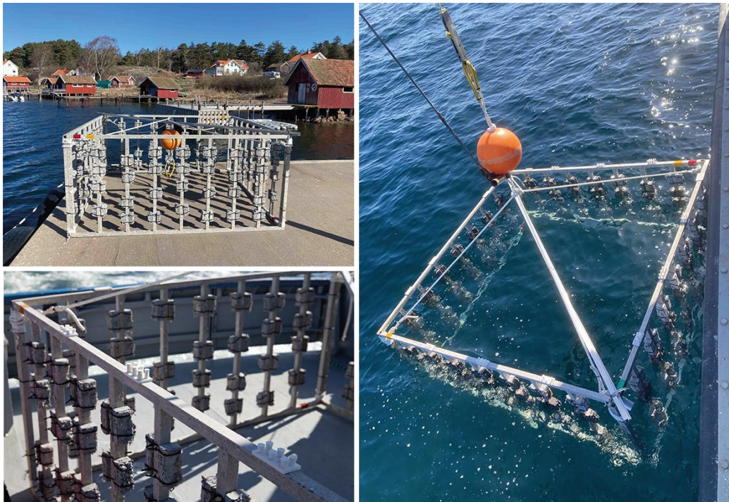
Figure 9: Settling panels with different cement mixtures, two surface structures (slag mixed with cement, and jute soaked in wet cement), and 3D printed complex substrates. Day of deployment, April 11, 2022.
