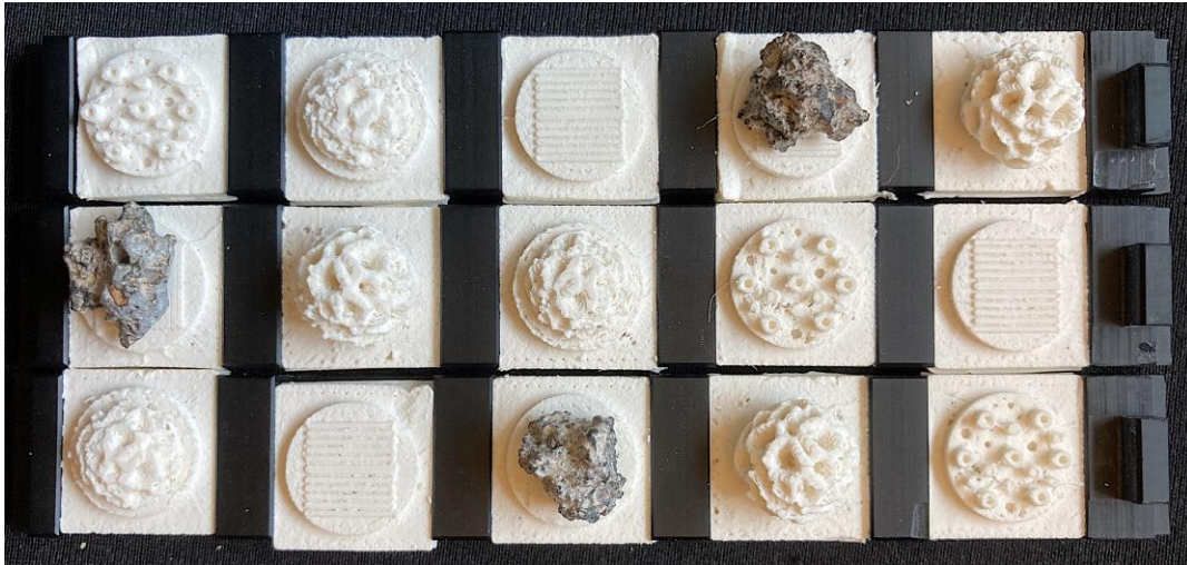
Fig. 1. Examples of surface structures of 3D printed substrates (here only LayBrick) and pieces of metallurgic slag. From top left: pillars, flat (low relief) Voronoi, ridges, slag, high Voronoi.
