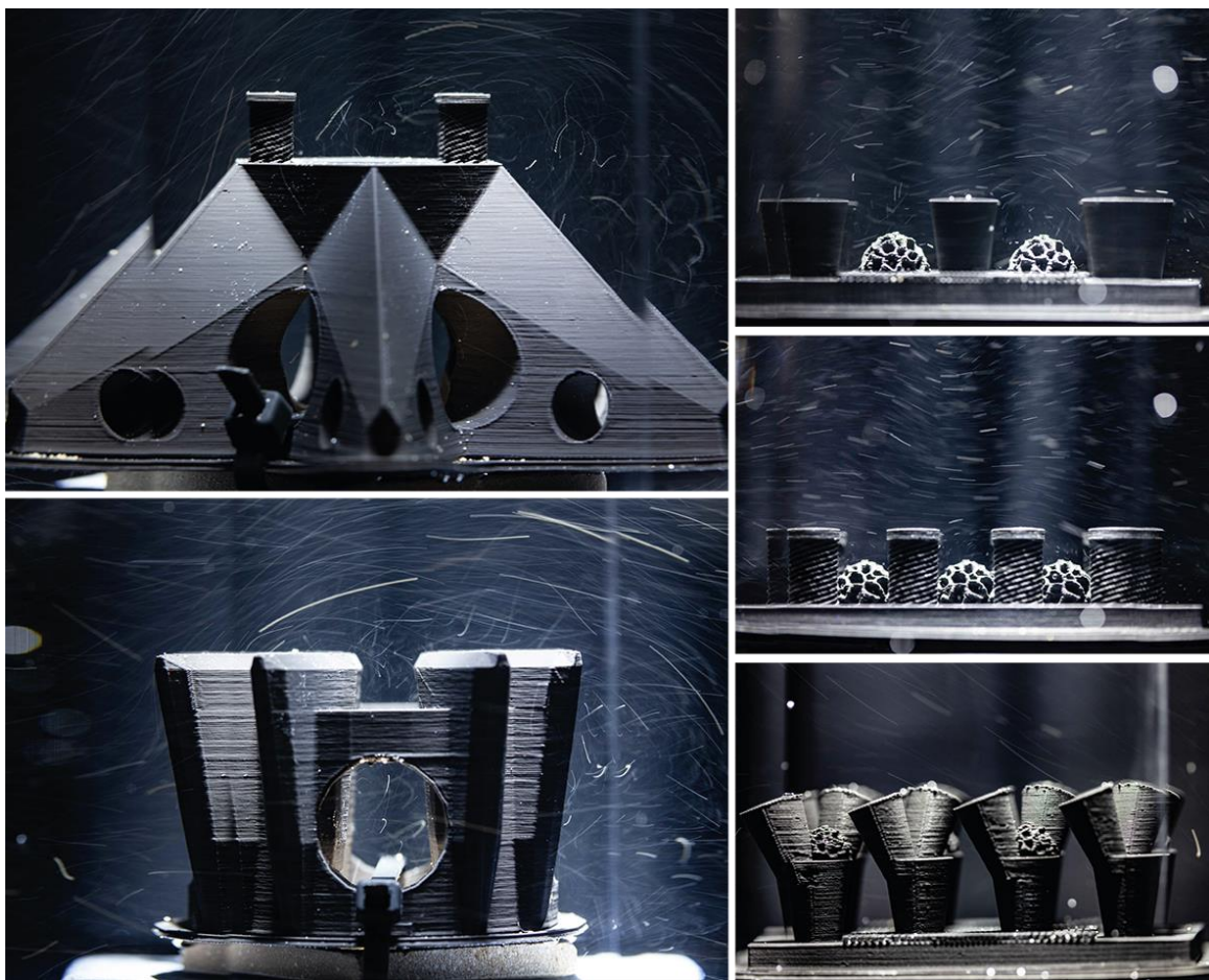
Figure 4. Examples of two of the six tested AR models (left) and three of the sixteen complex substrates (right) designed to enhance coral larval recruitment. The traces are particle movements over the substrates, achieved by long exposure time. Two velocities were used, 10 and 20 rpm. Images are taken in the small circular flume for the purpose of initial screening of AR models and substrates. The most promising ones will be further analyzed in the large flow channel equipped with a PIV system.
