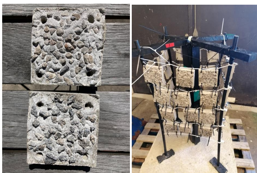
Fig. 7. Panels with added small stones, smooth slag, and porous slag, to test for the effect of chemical composition and porosity of the added material.
